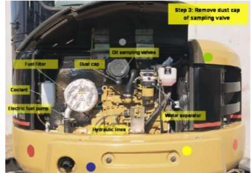
Recognition of open panel causes identification of components and instruction to remove cap
