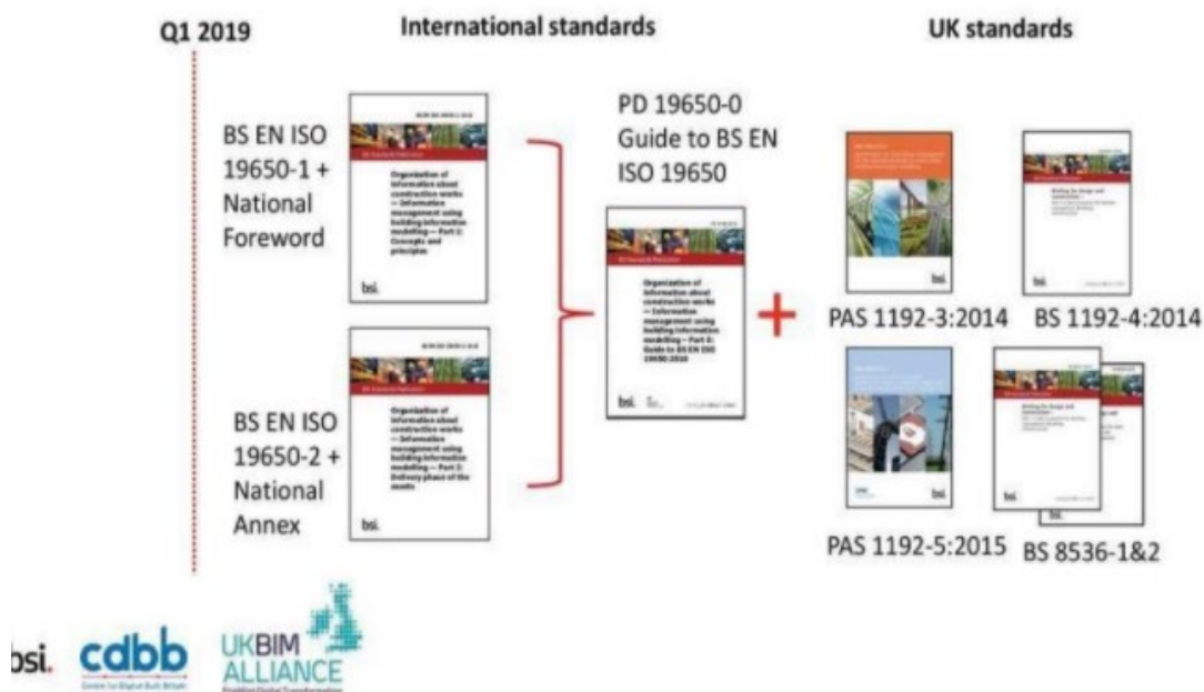
Figure 2: The UK BIM Standards, afterwards Q1 2019 (Source: cdbb, Center for Digital Built Britain, 2019)
