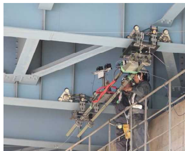
Bridge girder Suspended-types (Compound eye-type camera)
